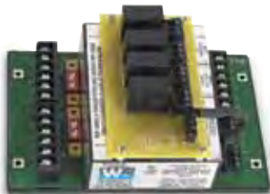
Warrick® Series 47 4-channel relay alarm panel control
